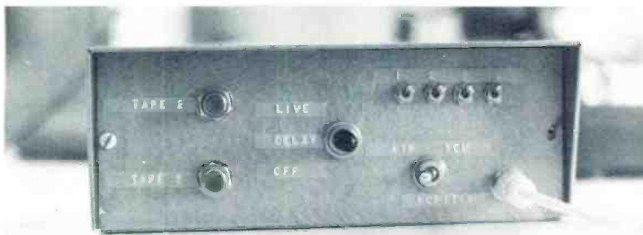
Photo #3 Delay system control panel.
